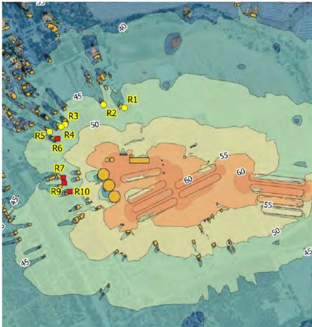
Figure F: Scenario C: Rail silo loading by conveyor –LA 10 dB
