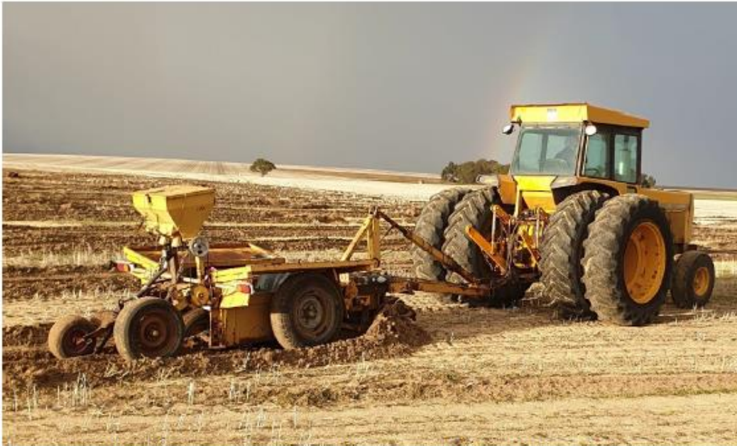
Photo 2: V-blade scalping, ripping and direct seeding with Chatfield Tree Planter, Jock's Camp compartment.
