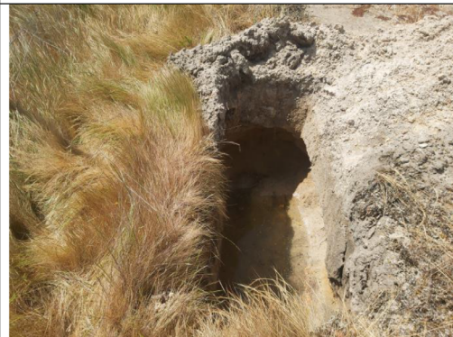
Photo 10: Soil Profile at Test Pit 9 (TP9)- land reserve area, Groundwater observed at 0.8m depth
