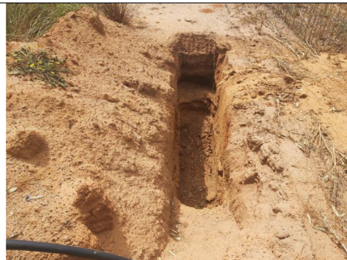
Photo 3: Soil Profile at Test Pit 1 (TP2)- Block F, Groundwater not observed
