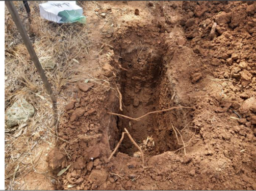
Photo 2: Soil Profile at Test Pit 1 (TP1)- Block G, Groundwater not observed
