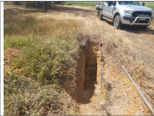
Photo 7: Soil Profile at Test Pit 5 (TP5)- Block C, Groundwater not observed
