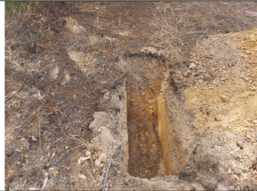
Photo 6: Soil Profile at Test Pit 4 (TP4)- Block D, Groundwater not observed
