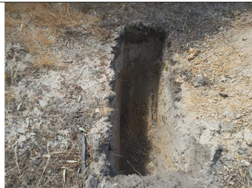
Photo 4: Soil Profile at Test Pit 3 (TP3)- Block E, Groundwater not observed
