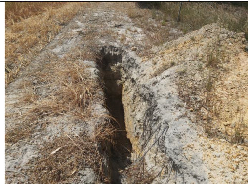
Photo 12: Soil Profile at Test Pit 8 (TP8)- Block H, Groundwater not observed
